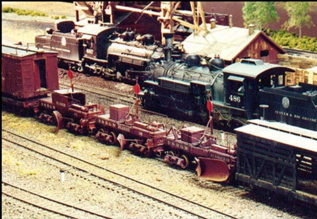
Here are three flangers, OF, OI and OB in storage in Chama. All have steel frames.
