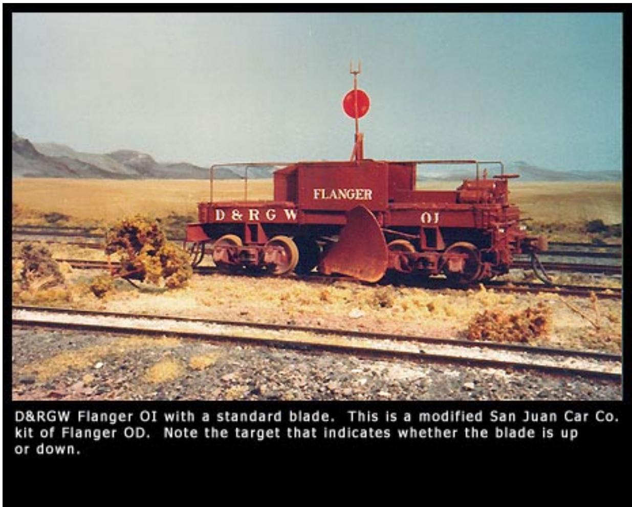
D&RGW Flanger OI with a standard blade. This is a modified San Juan Car Co. kit of Flanger OD. Note the target that indicates whether the blade is up or down.
